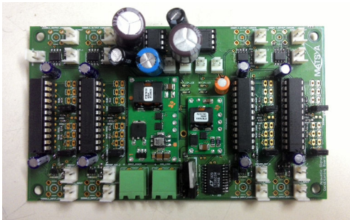
Figure 12: Custom Designed Acoustic board
