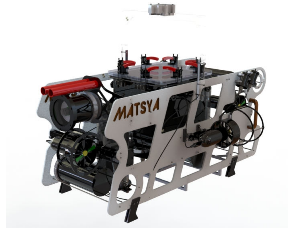
Figure 5: SolidWorks rendering of CAD model of Matsya
